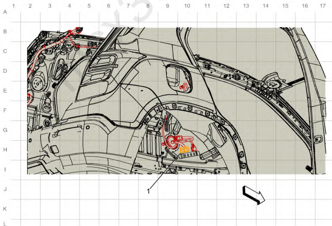
Fig. 47: Body Harness Routing - Right Rear Exterior (Trax). Courtesy of GENERAL MOTORS COMPANY
